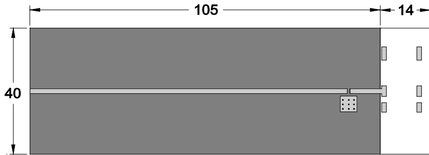
Fig. 2 Outlook and dimension of evaluation board
