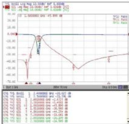
1608 / 2.45GHz Bluetooth /WLAN Band Pass Filter CFL4111715012454K
