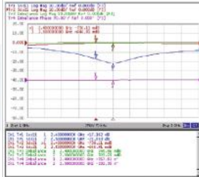
2012 / 2.45GHz Bluetooth/WLAN Balun CBA4711 714 00 2454K
