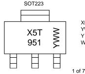
X5T 951 = Product Type Marking Code YWW = Date Code Marking Y or  $\overline{Y}$  = Last Digit of Year (ex: 5= 2015) WW or  $\overline{W}W$  = Week Code (01~53)
