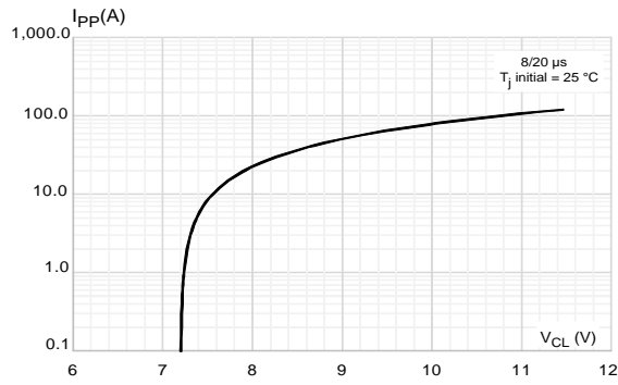
Figure 5: Peak pulse current versus clamping voltage (maximum value)
