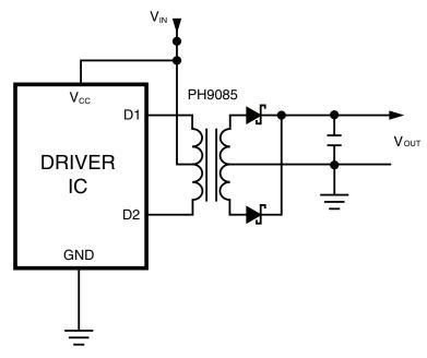
For a fixed 50% duty cycle mode of operation, the output voltage is simply determined by the input voltage and turns ratio. So, with the available turns ratios, a variety of output voltages can be selected.
