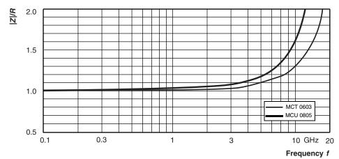
Relative impedance for 49.9  $\Omega$  chip resistor
