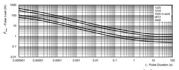
Maximum pulse load, single pulse; applicable if  $\bar{P} \to 0$  and n < 1000 and  $\hat{U} \le \hat{U}_{max}$ ; for permissible resistance change equivalent to 8000 h operation
