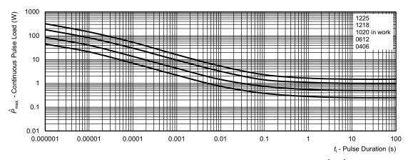
Maximum pulse load, continuous pulses; applicable if  $\bar{P} \leq P\left(\vartheta_{\rm amb}\right)$  and  $\hat{U} \leq \hat{U}_{\rm max}$ ; for permissible resistance change equivalent to 8000 h operation
