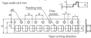
Taping condition: Lack of products in the middle of taping should be one MAX, but total quantity specified in the
