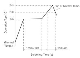
st Reflow temperature may vary by location even in the same reflow condition. Please check the reflow temperature at terminals and at the top of a switch to make sure the both temperatures are withiin the specification. If even one of them is out of the specifications, please adjust.
