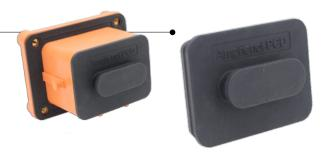
MINI MSD М 350 F Shell type: M: Plug F: Receptacle Fuse rating current: **XXX:** 080, 100, 125, 160, 200, 250, 315, 350, 400 (Unit: AMP) 000: No fuse needed, can directly use the terminal Fuse brand (this applies to plugs): /: Bussmann (by default) 1: Other brands (TBD) Flange mounted type (this applies to sockets): **F:** Front mounted R: Rear mounted
