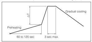
$\triangle T$ : Allowable temperature difference  $\triangle T \le 150$  °C
