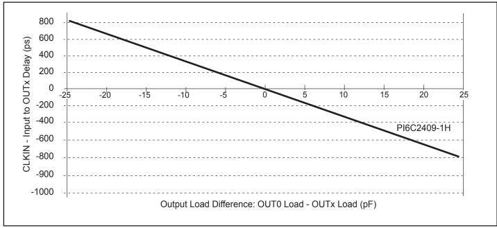
The relationship between loading of the OUT0 signal and other outputs determines the input-output delay. Zero delay is achieved when all outputs, including feedback, are loaded equally.
