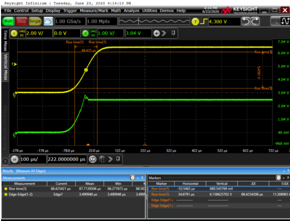
Figure 7. Power Up, 100µs, V_{BIAS}=6.5V , R_{BIAS}=2.5K
