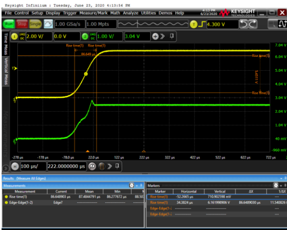
Figure 9. Power Up, 100µs, V_{BIAS}=6.5V , R_{BIAS}=20K
