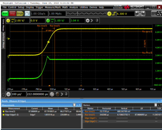
Figure 5. Power Up, 100 \mu s, V_{BIAS} =6.5V, R_{BIAS} =0.5K
