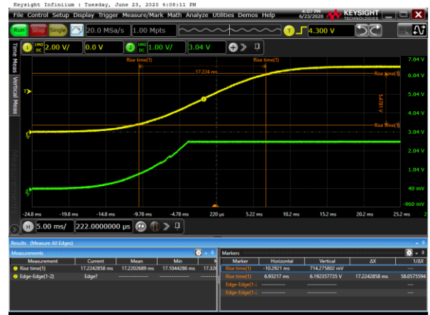
Figure 8. Power Up, 15ms, V_{BIAS}=6.5V , R_{BIAS}=2.5K
