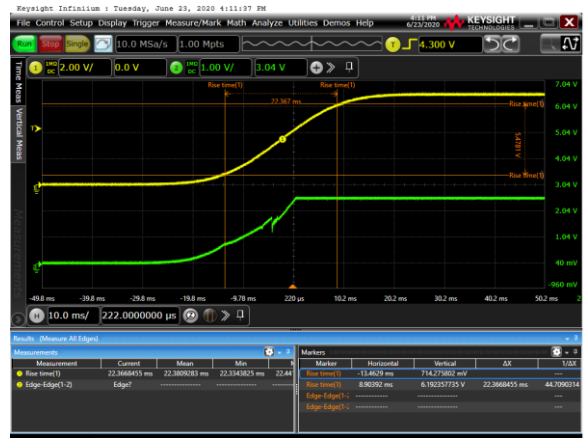
Figure 10. Power Up, 15ms, V_{BIAS}=6.5V , R_{BIAS}=20K
