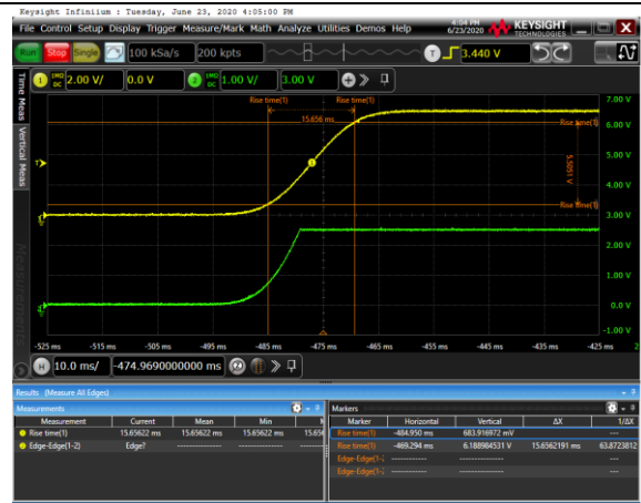
Figure 6. Power Up, 15ms, V_{BIAS} =6.5V, R_{BIAS} =0.5K
