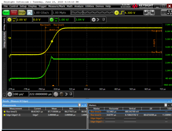
Figure 7. Power Up, 100 \mu\text{s} , V_{BIAS} = 6.5\text{ V} , R_{BIAS} = 2.5\text{ k}\Omega
