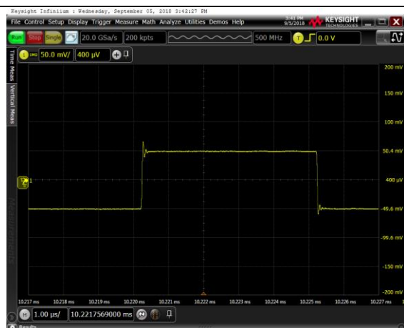
Figure 17. 100mV Signal Step Response
