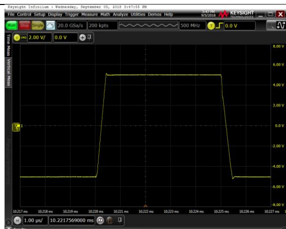
Figure 18. 10V Signal Step Response
