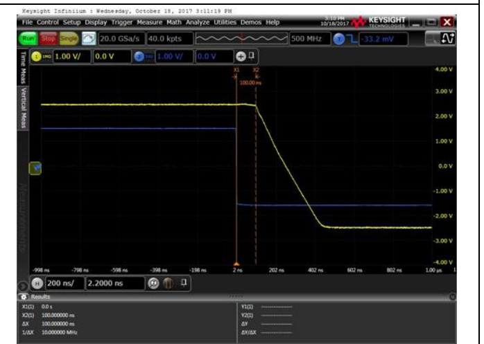
Voltage: 1V/div, Time: 200ns/div V_s = 5V , V_{IN} = 2V , R_L = \text{Open} , G = 3 Figure 24. Negative Overload Recovery
