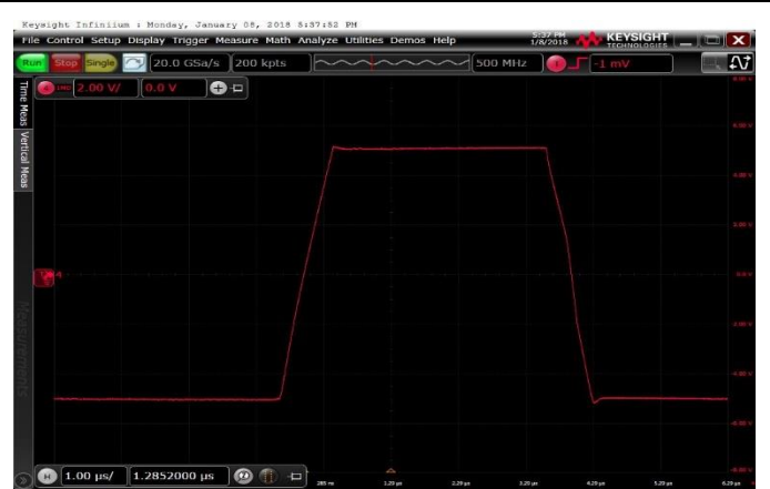
Voltage: 2V/div, Time: 1μs/div V_S = \pm 15V , R_L = 2K , C_L = 100pF , G = 1 Figure 26. 10V Signal Step Response
