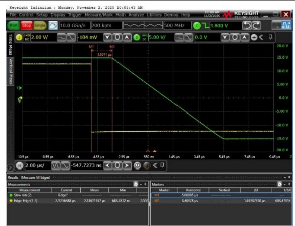
Voltage: 5V/div for Output, Time: 2us/div G=10, VREF = GND; VIN=10VPP, Load R=10K C=100pF Figure 22 Negative Overload Recovery
