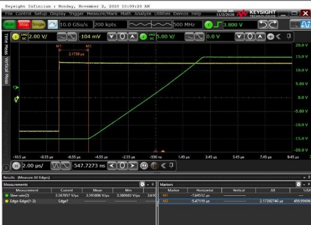
Voltage: 5V/div for Output, Time: 2us/div G=10, VREF = GND; VIN=10VPP, Load R=10K C=100pF Figure 21 Positive Overload Recovery
