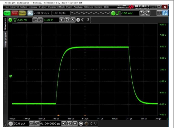
Voltage: 2V/div for Output, Time: 50us/div G=1000, VREF = GND; VIN=10mVPP, Load R=10K C=100pF Figure 26 Large-Signal Pulse Response
