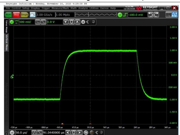
Voltage: 500mV/div for Output, Time: 50us/div G=10, VREF = GND; VIN=2mVPP, Load R=10K C=100pF Figure 30 Small-Signal Pulse Response
