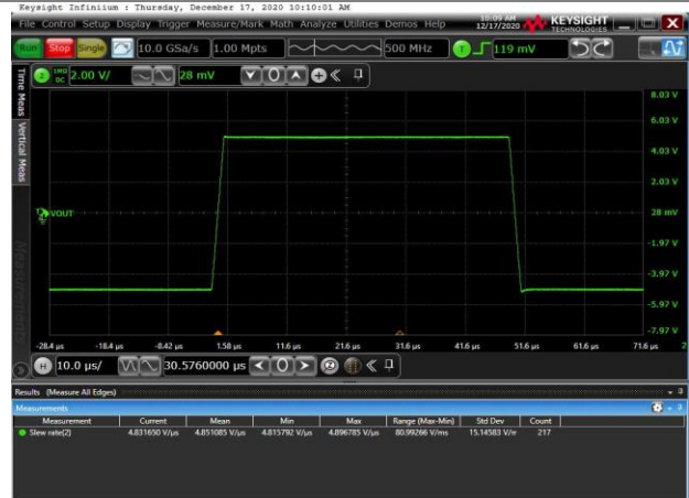
Voltage: 2V/div for Output, Time: 10us/div G=1, VREF = GND; VIN=10VPP, Load R=10K Figure 20 Slew Rate
