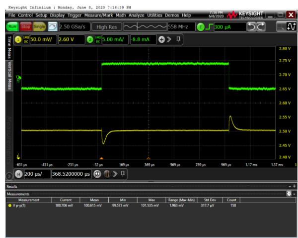
Figure 12. Load Transient, \pm 5\text{ mA} , V_{IN} = 2.8\text{ V} , C_{IN} = 1\ \mu\text{F} , C_{OUT} = 1\ \mu\text{F} , 50 mV/div
