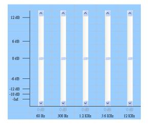
User can adjust a variety of sound effects according to requirement; the results will be stored in EEPROM after adjustment, and it can use single button to change different sound effect in cycle approach, simultaneously, also provide a single LED for indication of ON/OFF sound effect. By default, SSS1700 built-in a subwoofer sound settings, therefore, under no external EEPROM case, there is still an EQ sound transformation for user. Preset bass (SUBWOOFER) sound settings are as follows:
