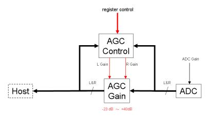
AGC parameter setting can be set in EEPROM. The control features include stability of time, error range, active manner, hold time, speed adjusting and son on, these parameters need for individual settings. Its operational diagram refers as below:
