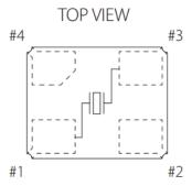
Pin #1: Crystal Pin #3: Crystal Pin #2: GND (\*)
