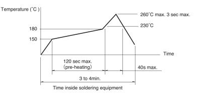
TACT Switch™ Soldering Conditions
