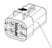
4 POS, PLUG, SOCKET, NORMAL SEAL, ATP SERIES
