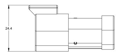
NOTES: UNLESS OTHERWISE SPECIFIED 1. MATERIAL: HOUSING: THERMOPLASTIC SEAL: SILICONE RUBBER
