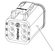
PLUG, 6 SOCKET, AT SERIES, REDUCED DIA. WIRE SEAL
