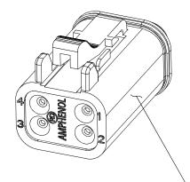
PLUG, 4 SOCKET, AT SERIES, REDUCED DIA. WIRE SEAL
