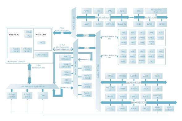
The AXI Crossbar of the MCU bus is a bus matrix used to interconnect the CPU core
