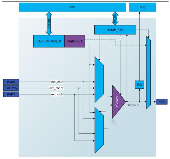
The blue part is a digital circuit, and the purple part is an analog circuit.
