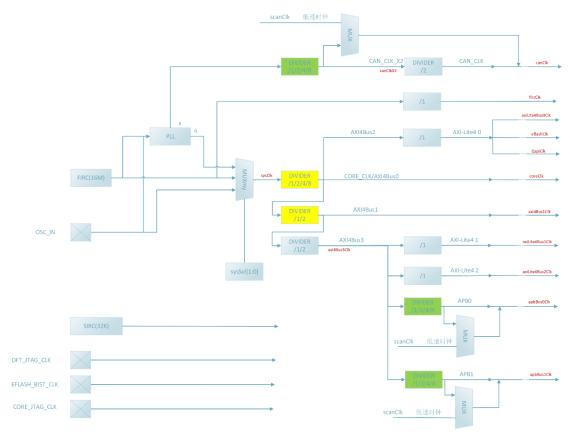
The clock management module provides clock selection for MCU. It includes fast internal clock (FIRC), internal slow clock (SIRC), external crystal oscillator (OSC) and PLL as the clock source. The reference clock of PLL can be derived from FIRC or OSC.
