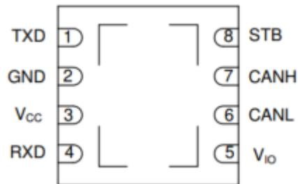
Figure 1 Pin distribution of FD CAN chip
