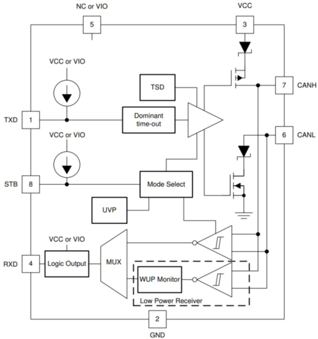
Figure 2 Block diagram of internal circuit structure
