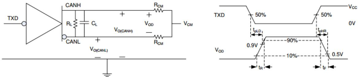
Figure 3 FDCAN transmit test circuit and timing diagram
