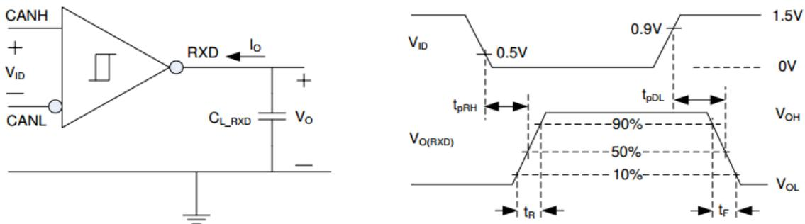
Figure 4 FDCAN receiving test circuit and timing diagram
