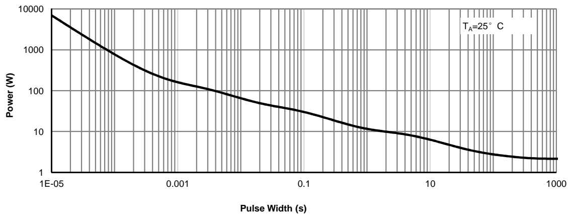
Figure 14: Single Pulse Power Rating Junction-to-Ambient (Note H)
