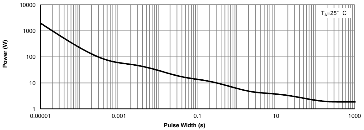
Figure 14: Single Pulse Power Rating Junction-to-Ambient (Note H)
