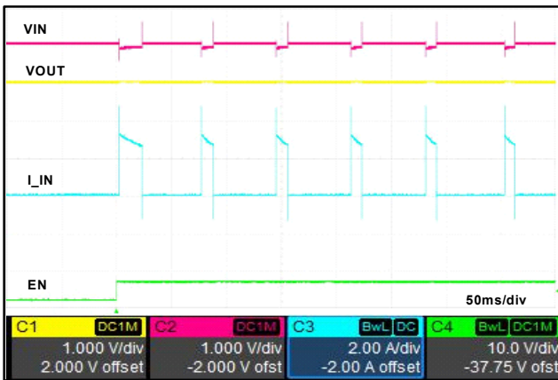
Figure 9. Starting Up into Shorted Output
