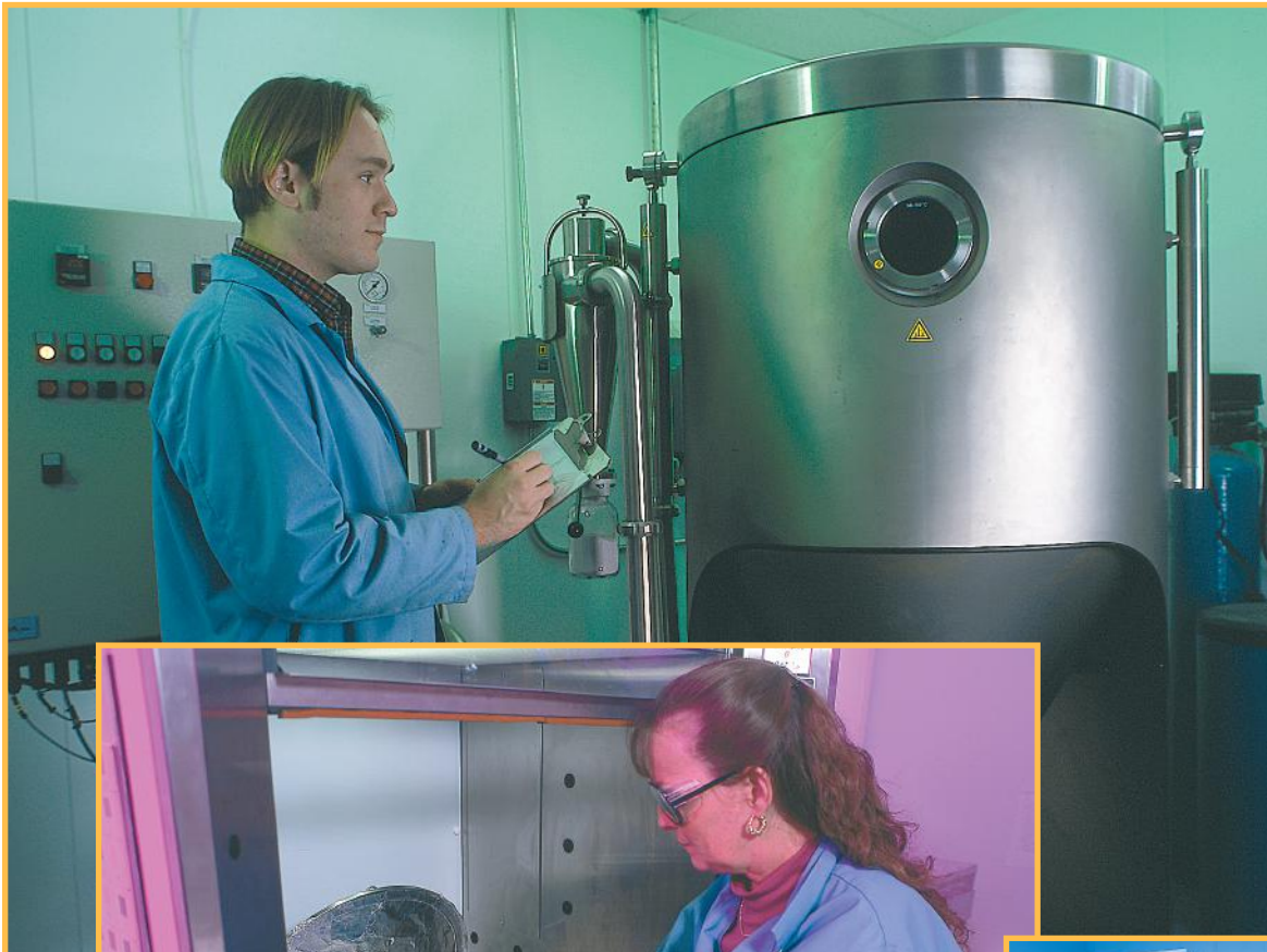
◀ Niro Spray Dryer - Spray drying is a unique drying process involving both particle formation and drying
