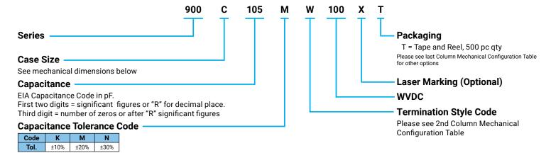
The above part number refers to a 900 C Series (case size C) 1.0 MFd capacitor, M tolerance (±20%), 100 WVDC, with W termination (Tin/Lead, Solder Plated over Nickel Barrier), laser marking and ATC Matrix Tray packaging.
