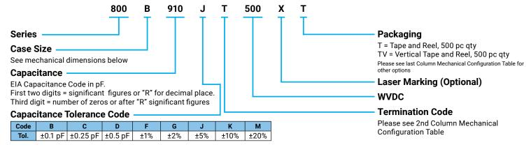
The above part number refers to a 800 B Series (case size B) 91 pF capacitor, J tolerance (±5%), 500 WVDC, with T termination (Tin Plated over Nickel Barrier Termination, RoHS Compliant), laser marking and tape and reel packaging.
