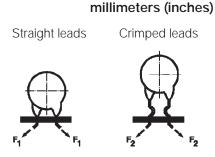
Maximum pull force during insertion and lead cut
