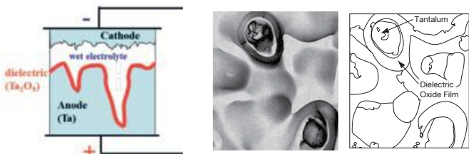
Figure 1 a. Basic Tantalum Wet Electrolytic Capacitor System
