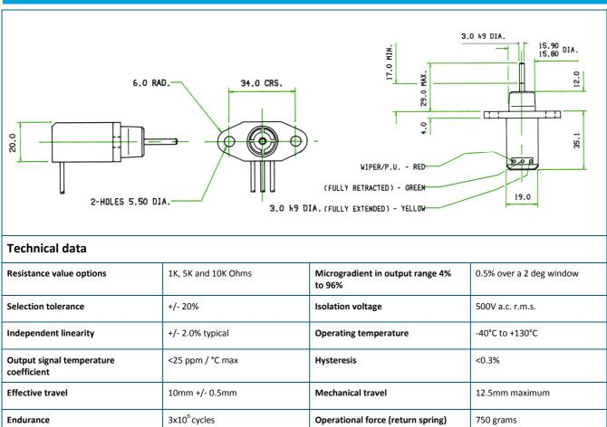
Conductive polymer potentiometer with 10mm linear effective travel for automotive and industrial applications. Connection via flying leads colour coded as detailed below, 200 mm in length. Standard spindle is 3mm diameter with a length of 29mm from fixing-face., but other lengths area available upon request
