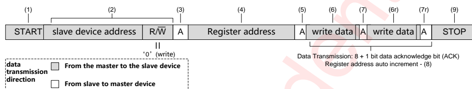
Figure 32 Writing process (data transmission direction remains the same)
