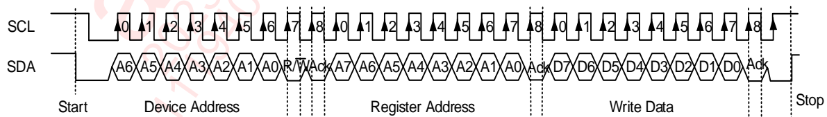
Figure 6 I 2 C write byte cycle
