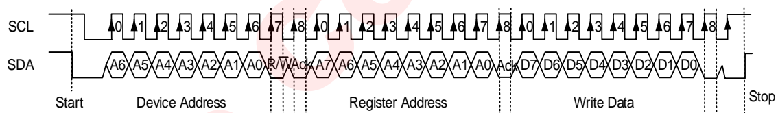
Fig 34 I 2 C Write Timing
