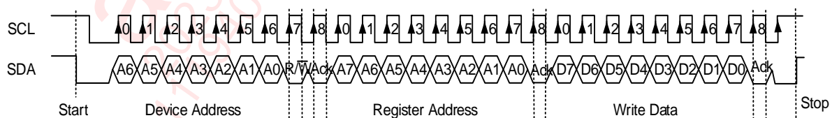
Figure 6 I 2 C write byte cycle
