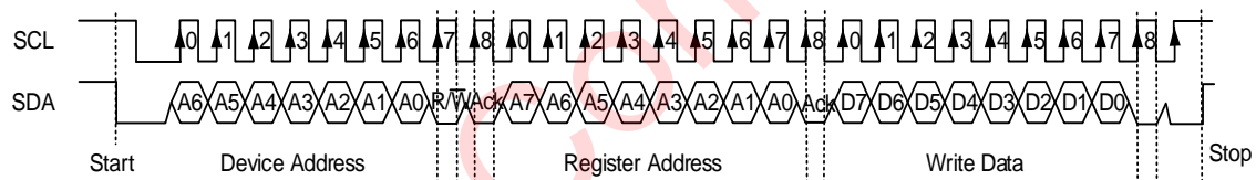
Fig 27 I 2 C Write Timing
