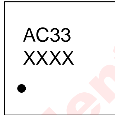
AC33 - AW2033DNR XXXX - Manufacture date code
