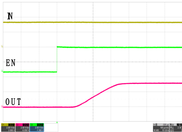
C1: 2.00V/div C2: 2.00V/div t=160μs/div C4: 2.00V/div VIN=3.3V, CIN=1μF, COUT=1μF, Rload=5Ω
