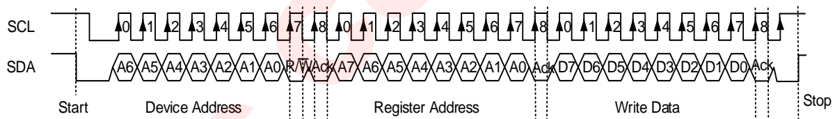
Figure 9 I 2 C Write Byte Cycle
