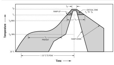
Ramp-up rate = 3 °C/sec. max. Ramp-down rate = 6 °C/sec. max.  $T_L = 217$  °C  $t_L = 60-150$  sec.
