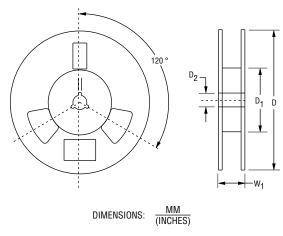
Devices are packed as shown here in compliance with EIA-481-C standard.
