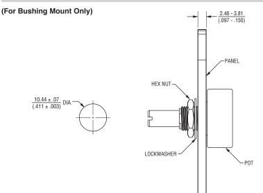
Panel thickness and hole diameters are recommended for best fit. However, customers may adjust the dimensions to suit their specific application.
