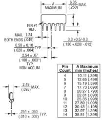
Maximum package length is equal to 2.54mm (.100") times the number of pins, less .005mm (.002").
