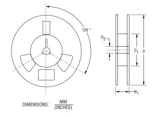
Devices are packed as shown here in compliance with EIA-481-C standard.
