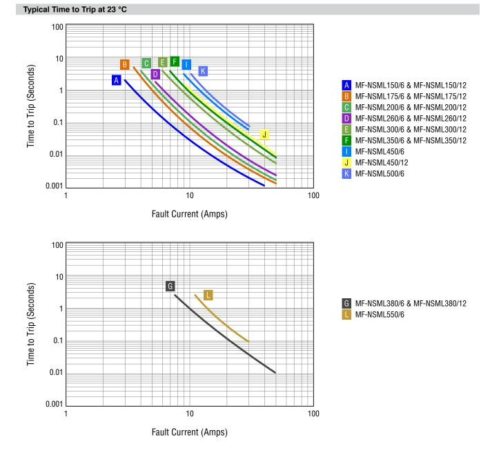
The Time to Trip curves represent typical performance of a device in a simulated application environment.
